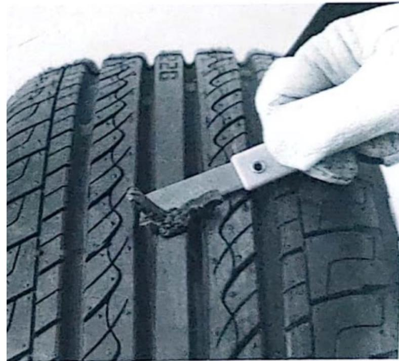
6. Use the included knife to trim excess plug material and re-inflate tire recommended pressure.
