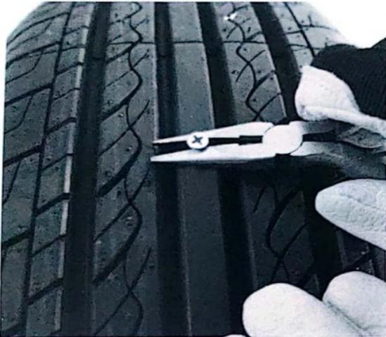
1.Remove offending object from tire with included heavy duty pliers.
