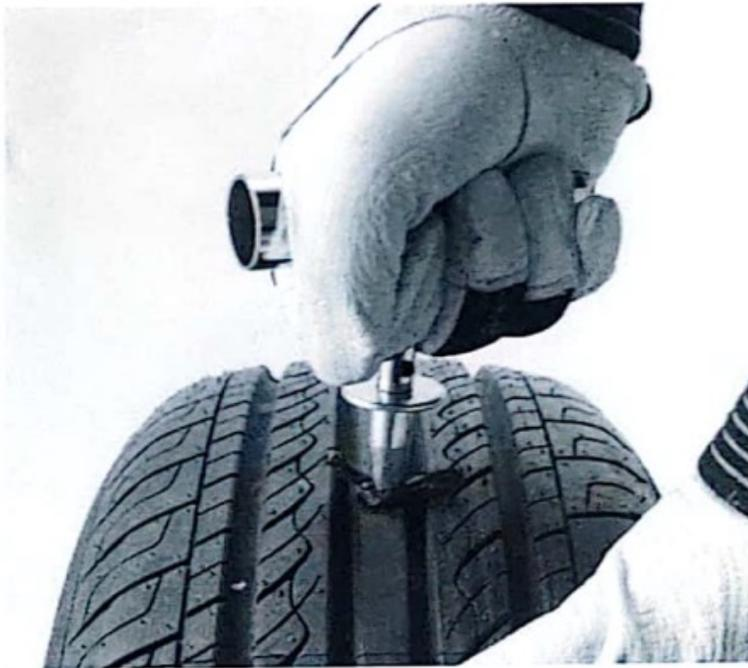
5. Slide the retaining platform until against the tire. Hold the retaining platform against the tire while quickly and firmly pulling the T-handle up leaving the plug in place.
