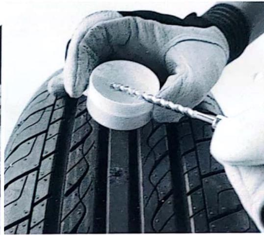
2.Apply lubricant to the spiral shaft of the reamer tool. This will help to probe the hole and temporarily separate the steel belts.
