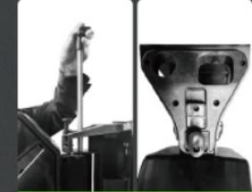
Disassemble the washer body
